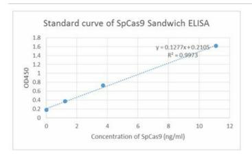
Standard curve of SpCas9 Sandwich ELISA. The SpCas9 Sandwich ELISA assay is developed by using GenCRISPR™ SpCas9 Antibody (14B6) (GenScript, A01936-40) and GenCRISPR™ SpCas9 Antibody (4A1) (GenScript, A01935-40) as capture and detection antibody, respectively. These two antibodies recognize different epitopes.
